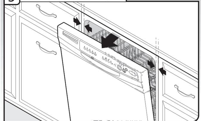
Open door and check that space between dishwasher cabinet opening and tub is equal on both sides. If spacing is not equal, loosen bracket screws secured and shift tub. Tighten bracket screws.
